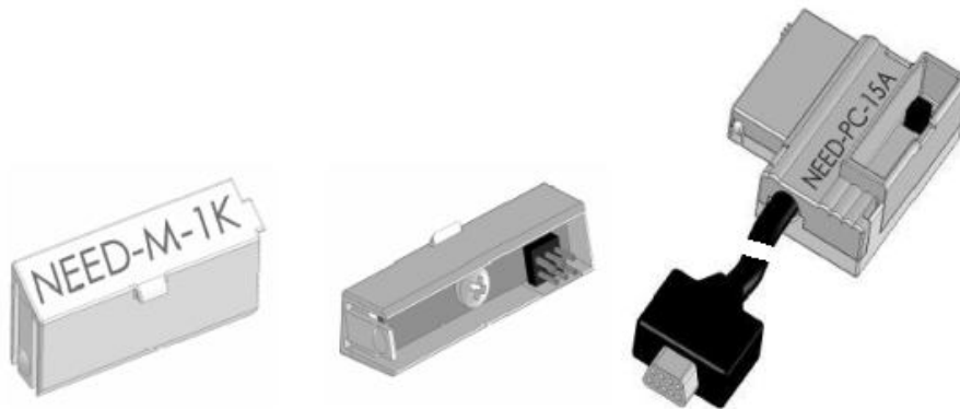
Fig. 2.3.2. Programming and diagnostics cable RS232 and memory with A type connector.
