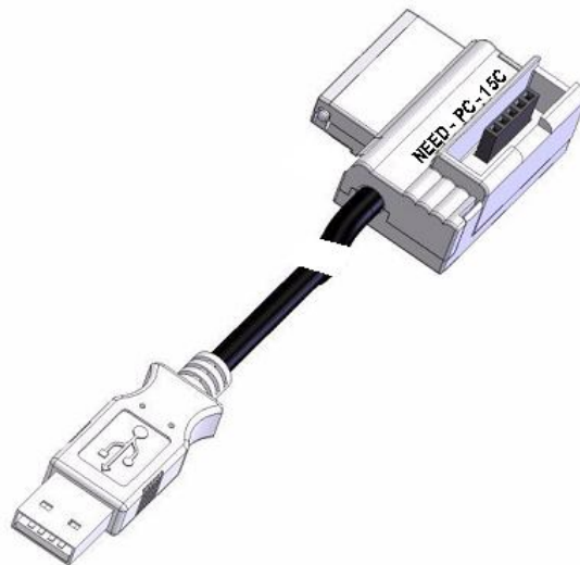
Fig. 2.3.4. Programming and diagnostics cable USB with B type connector.
