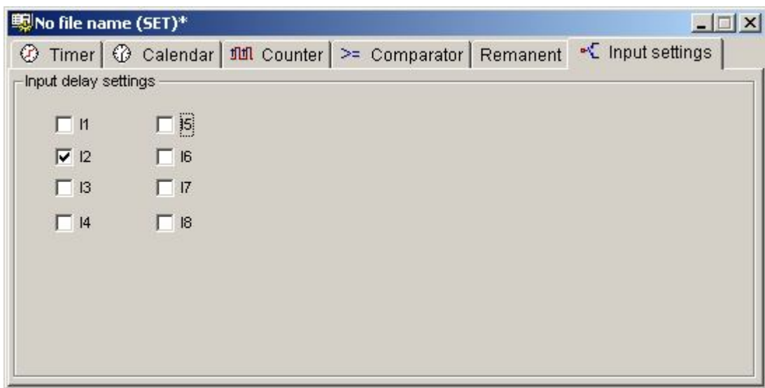
Fig. 8.4.2. Sample input delay configuration.
